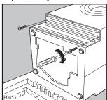
Set the machine upright and remove the two remaining bolts from the back.
